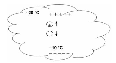
When lightning strikes, negative charge from the bottom of the cloud leaps down through the air to the ground. A lightning flash usually consists of several static discharges one after another. The temperature inside a flash can be around  $25\,000$  °C.
