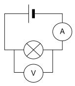
How will the ammeter and voltmeter readings change, if the bulb burns out?
