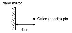
9.1 Draw a vertical line, 10 cm long, to represent the mirror. Draw a dot at a perpendicular distance of 4 cm from the mirror, to represent the office (needle) pin. Draw a ray from the dot so that the ray makes an angle of 55° with the mirror. Draw an accurate ray diagram showing the following:
